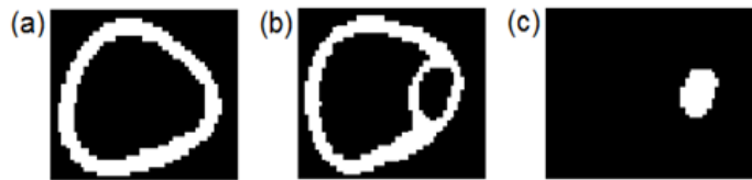
Fig. 3. (a) The healthy bone bar slice; (b) The defected bone bar slice; (c) The output difference between a and b
